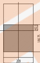
Dimension of Panel Cover Cutting - Handle Trip Unit Exposure
