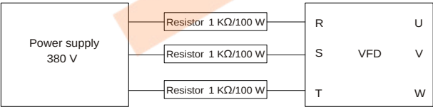
Figure 8–2 Charging circuit example of driving devices of 380 V
