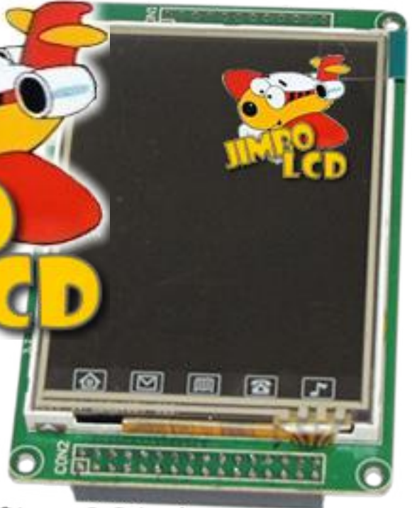
Size : 3.2 inch Resulation : 240*320 Driver : SSD1289
